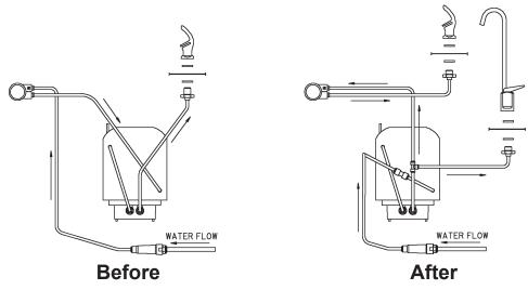
The water storage tank must be converted to a pressurized tank for the glass filler to operate properly. The tank is non-pressurized in a standard unit. The following steps detail how the water flow tubing is re-routed to create a pressurized tank and provide a supply line to the glass filler.
